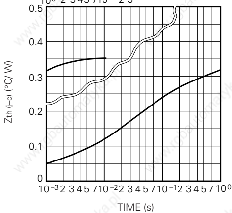
TRANSIENT THERMAL IMPEDANCE CHARACTERISTIC (TRANSISTOR)
