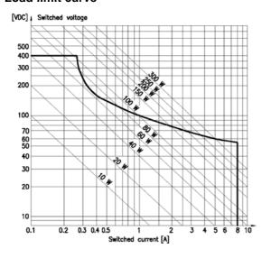
Loads in the range under the curve can be switched safely. The arc will extinguish before the opposite contact makes.
