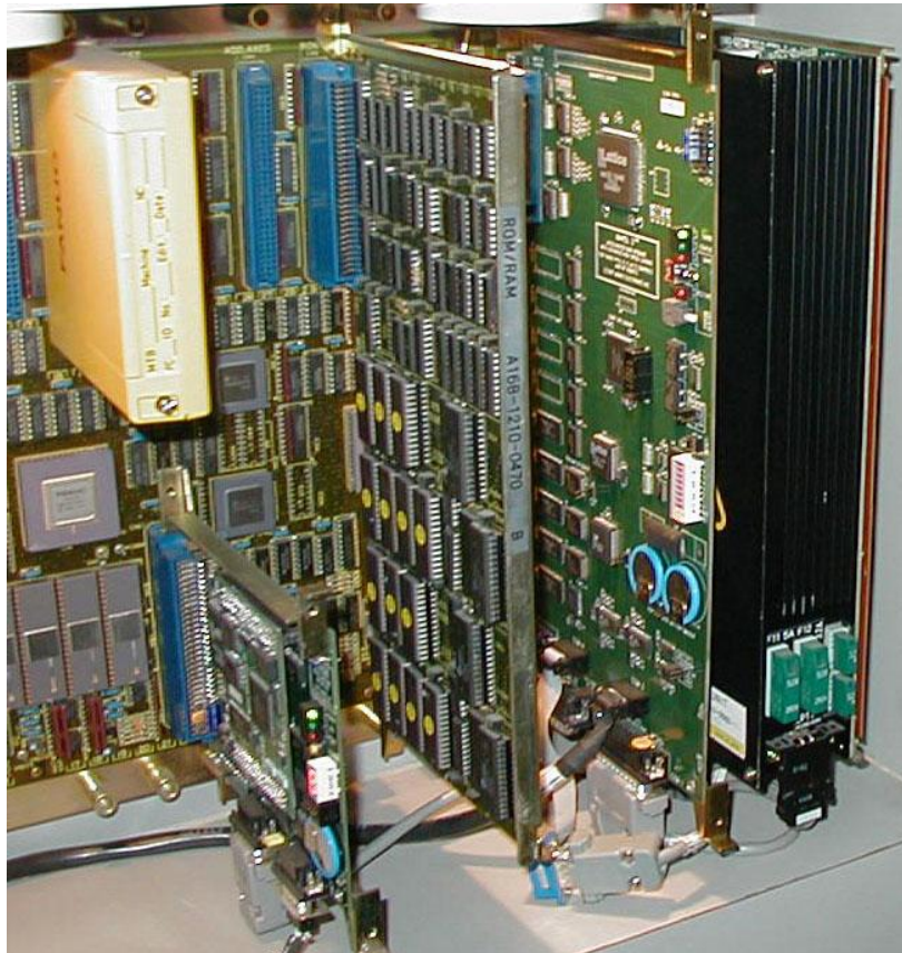
HSL3 Mounted in a Fanuc 11 with BMI board connected
