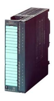
SIMATIC S7-300, DIGITAL MODULE SM 323, OPTICALLY ISOLATED, 16 DI AND 16 DO, 24V DC, 0.5A, AGGREGATE CURRENT 4A, 1X40 PIN
