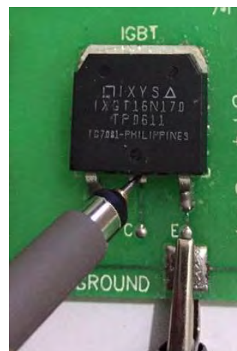
Figure 151: Channel1 Probe Used for Collector - Emitter Measurement
