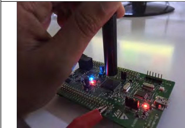
Figure 49: IR Sensor Component Temperature Measurement (Step 7)
