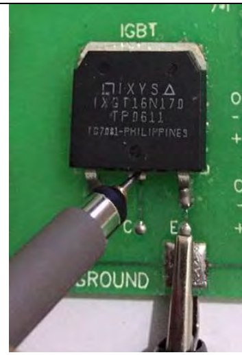
Figure 153: Channel1 Probe Used for Collector - Emitter Measurement
