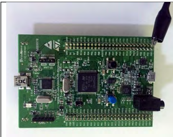
Figure 216: Connecting the Crocodile Probe Electronic Circuit Board Chassis (Step 1)
