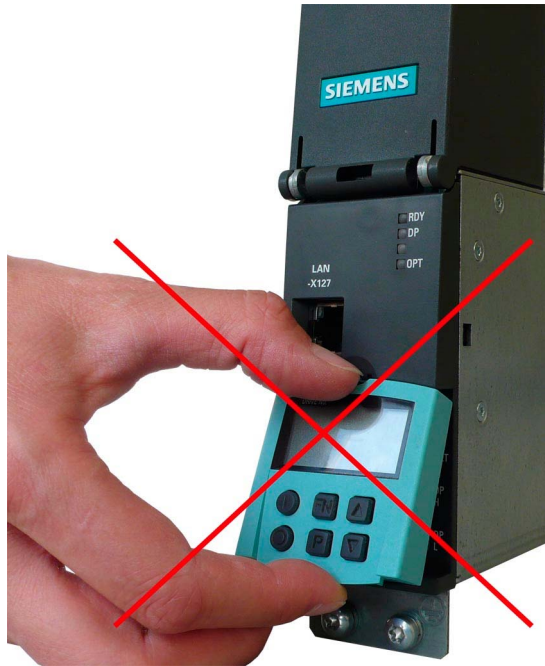
Figure 3-3 Incorrect removal of the BOP20 from a CU320-2 DP (example)
