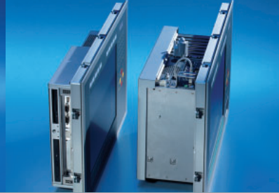
The Panel PCs CP6xxx are designed for installation in the front of a control cabinet.
