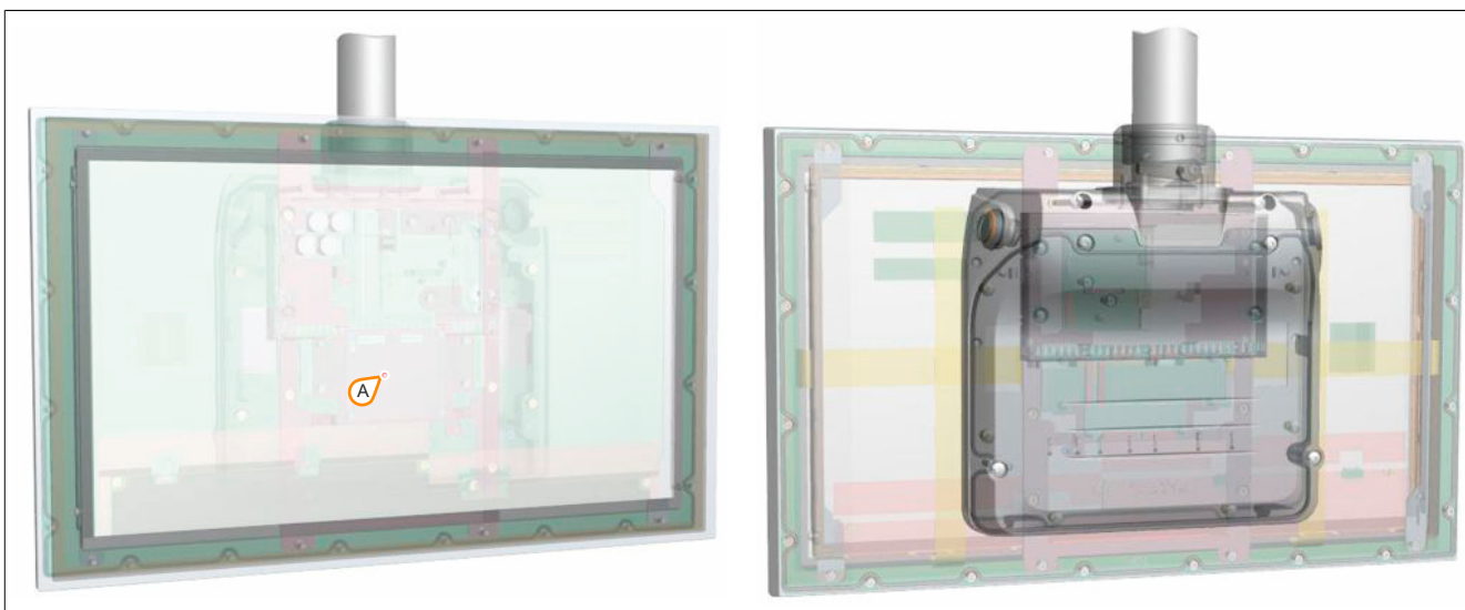
Figure 11: Automation Panel 5000 - Temperature sensor position
