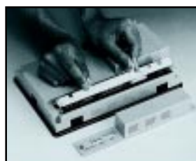
Replaceable backlight on LCD screen
