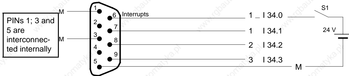
Figure 3-24. Connecting the Interrupt Inputs
