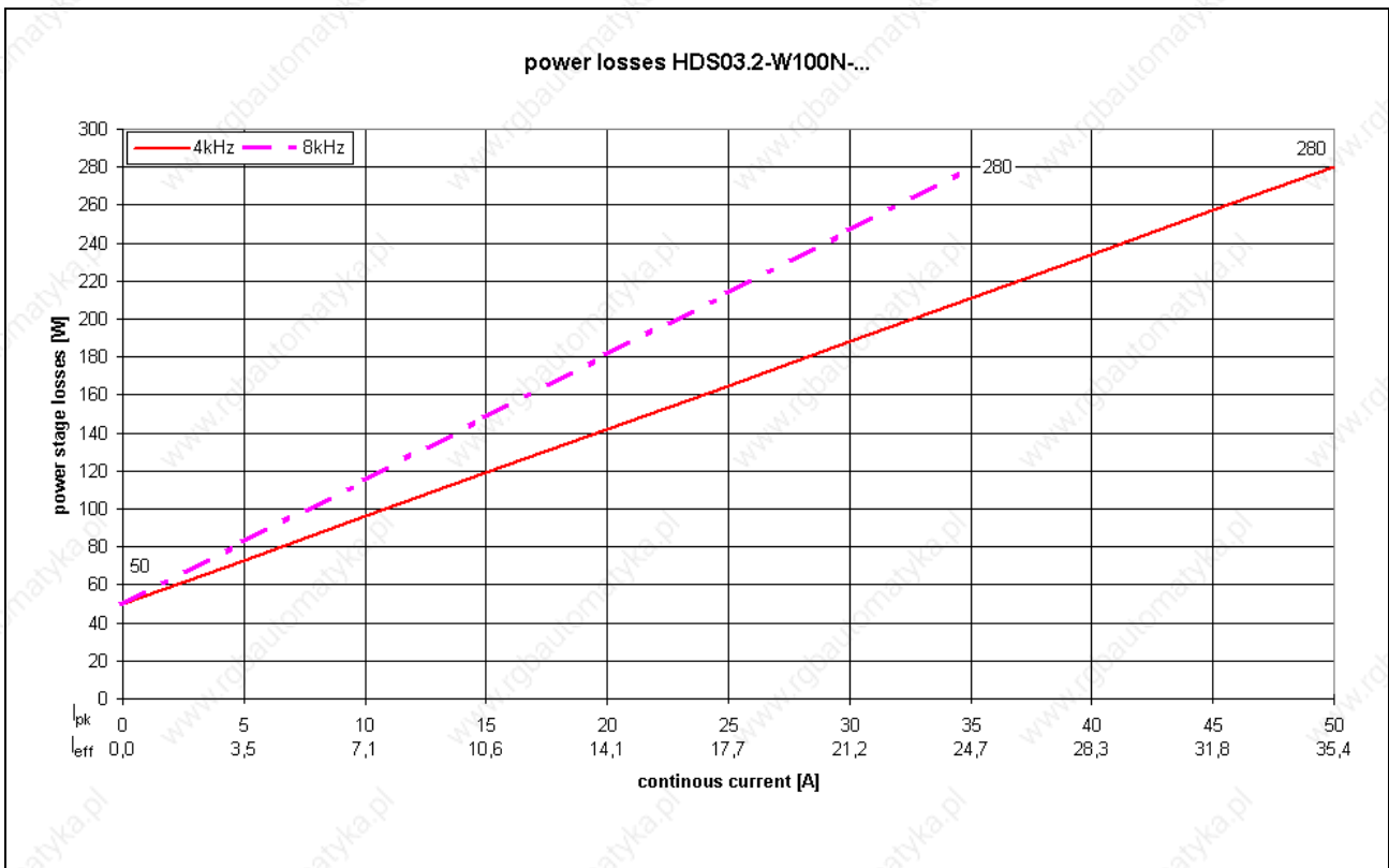
Fig. 7-4: Power loss HDS03.2W0100N-
