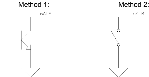
Fig. 2-1-4. Methods of the drive unit providing signals
