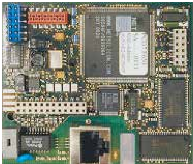
PCD7.F655 * Intelligent interface module for connection to Ethernet TCP/IP
