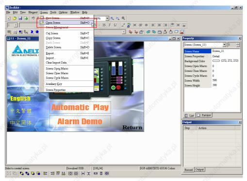
Fig. 2.7.6 Choosing Open Screen command from menu bar
