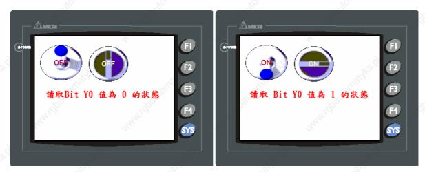
Fig. 3.2.2 Example of Button elements
