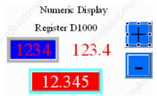
Fig. 3.2.6 Example of Increment / Decrement buttons
