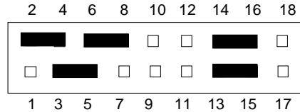
Configuration #5: 128K x 8 ROM/PROM/EPROM (Factory Configuration)
