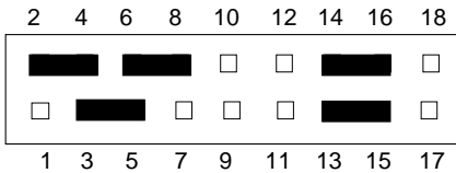
Configuration #5: 128K x 8 ROM/PROM/EPROM (Factory Configuration)
