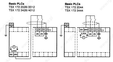
The fast response time of the event-triggered inputs 10,24 and 10,25, require the use of shielded cables for connecting these inputs.
