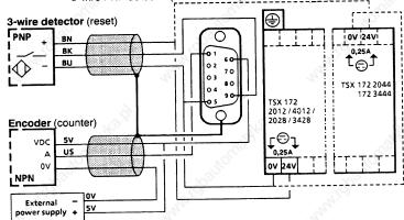
Example 2: Connecting a Telemecanique XCC-H..S.. encoder (counter) and a 3-wire PNP detector (used for reset).
