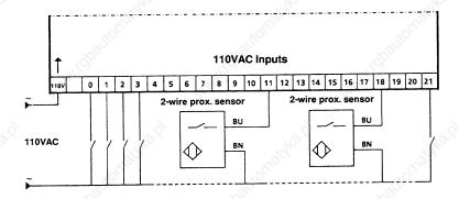
2-wire AC sensor: 110VAC rated supply.
