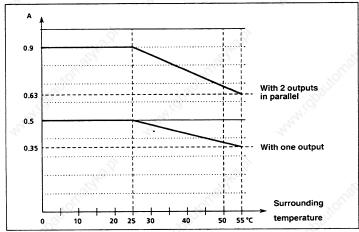
The I/O characteristics are given for a load rating of 60% (number of I/O at state 1 in relation to the total number of I/O).
