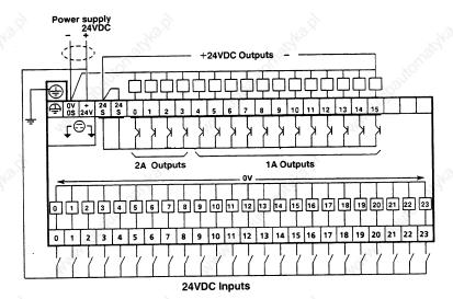
Notes: • The diagrams above and on the facing page, show a 24VDC power supply that is separate from that of the PLC and the inputs although it is possible to use the same supply. In all cases the 0V lines must be common.
