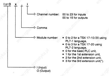
Addressing the event triggered inputs IO,24 and IO,25, available on TSX 17-20.
