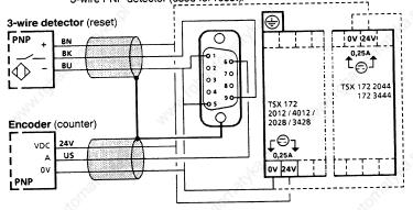
**Connection** is made to the top left (9-pin) female connector on the TSX 17-20. The connection is made using a TSX CCB 020 cable, length 2 meters, that is fitted with a (9-pin) male connector at one end, the other end can be fitted with a TSX CAC 04 (9-pin) connector that should be soldered on.
