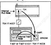
Transfer from the PLC RAM memory to the EPROM is always performed with the cartridge fitted in the TSX 17 ACC6 adaptor and controlled by the TSX T407 terminal in Transfer mode.
