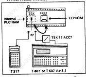
The transfer from the PLC RAM to EEPROM or from EEPROM to PLC RAM always takes place with the cartridge fitted in the PLC and the micro switch ① set to the Work position.
