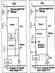
The Man/Auto switch allows the forcing of outputs when using a terminal connected to a PLC that is stopped (after SY8 is set to 0).
