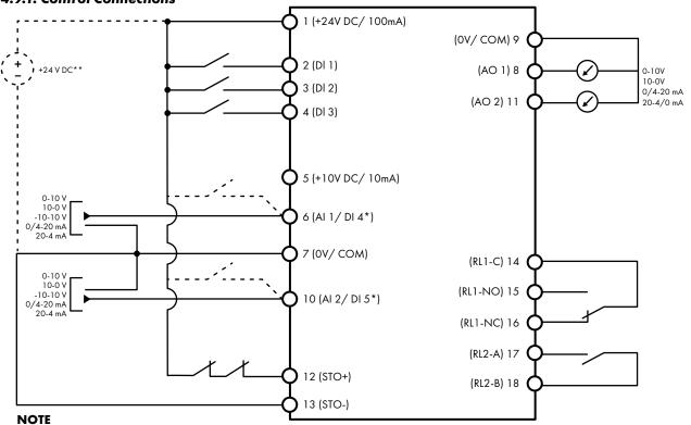
\* Dashed lines shows connection for analog inputs in digital mode
