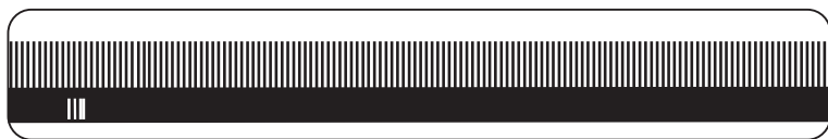
Scale with one reference mark
