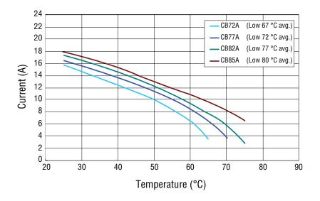
The above curves were derived from placing test samples in an oven at 25 °C, 40 °C, 60 °C and so on, increasing current flow through the sample at a rate of 0.1 A/minute and recording the current value when the sample trips.
