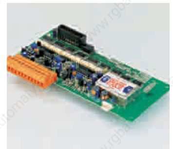
Analogue output board 2 outputs, 10bit resolution
