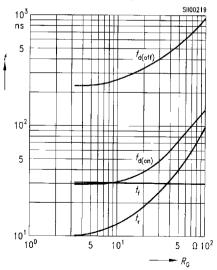
**Typ. switching time**  $t = f(I_{\rm C})$  Inductive load, parameter:  $T_{\rm J} = 125\,^{\circ}{\rm C}$   $V_{\rm CE} = 600\,$  V,  $V_{\rm GE} = \pm\,15\,$  V,  $R_{\rm G} = 22\,$   $\Omega$
