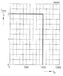
Safe operating area, short circuit  $I_{\rm C} = f\left(V_{\rm CE}\right), \, V_{\rm GE} = \pm \, 15 \, {\rm V}$   $T_{\rm I} \leq 150 \, ^{\circ}{\rm C}, \, t_{\rm SC} \leq 10 \, \, \mu{\rm s}, \, L < 50 \, \, {\rm nH}$
