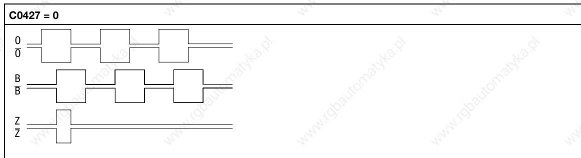
Fig. 3-59 Phase-delayed signal sequence (CW rotation)
