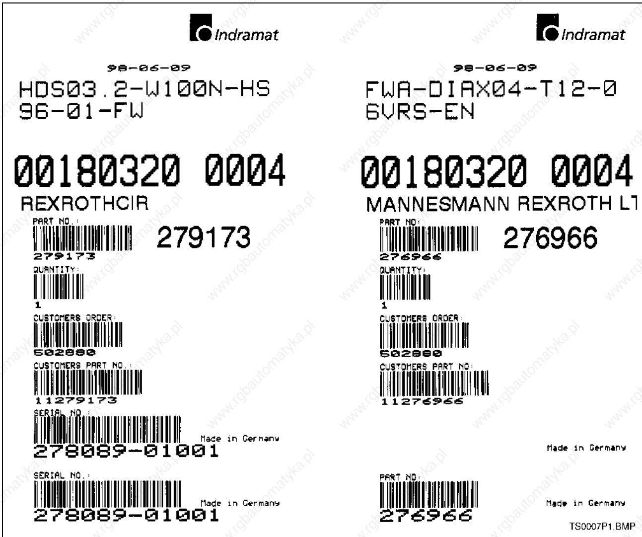
Fig. 10-1: Barcode sticker on the packaging of a HDD / HDS (Example)
