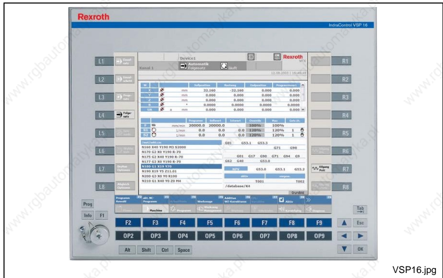
Fig. 5-1: VSP 16.1 with 12" color display
