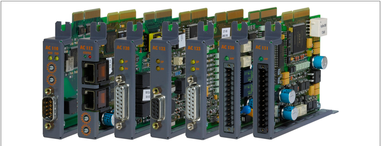
Figure 2: Plug-in modules allow optimized, application-specific configuration of ACOPOS servo drives
