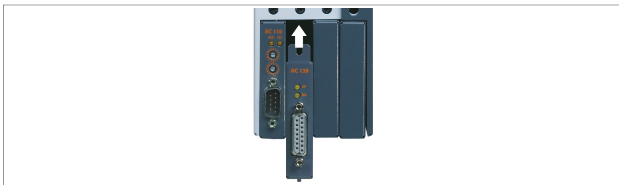
Figure 61: Installing ACOPOS plug-in modules
