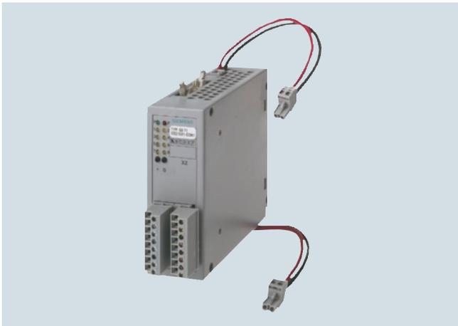
The interface module is used to connect 8 digital outputs with conversion of the 24 V DC voltage on the module side to a max. of 24/48 V DC/AC on the plant side using transistors.
