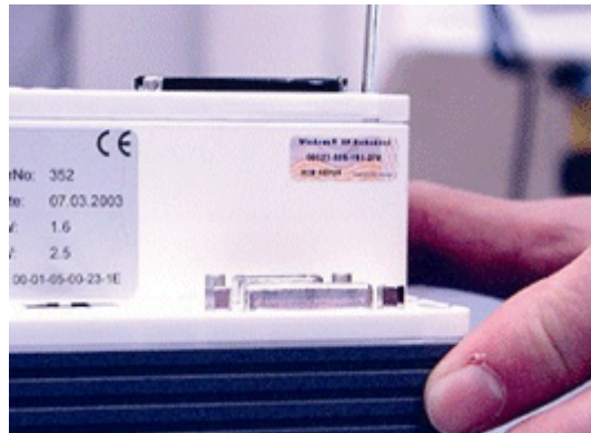
FIG1: Ejecting the CF card
