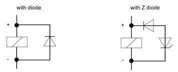
Diode/Zener diode circuits have the following characteristics:
