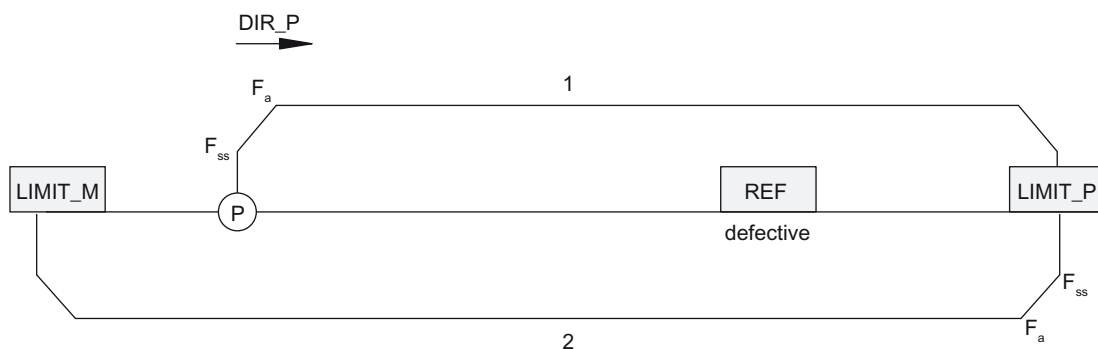
Figure 2-9 Defective reference cam, start before REF
