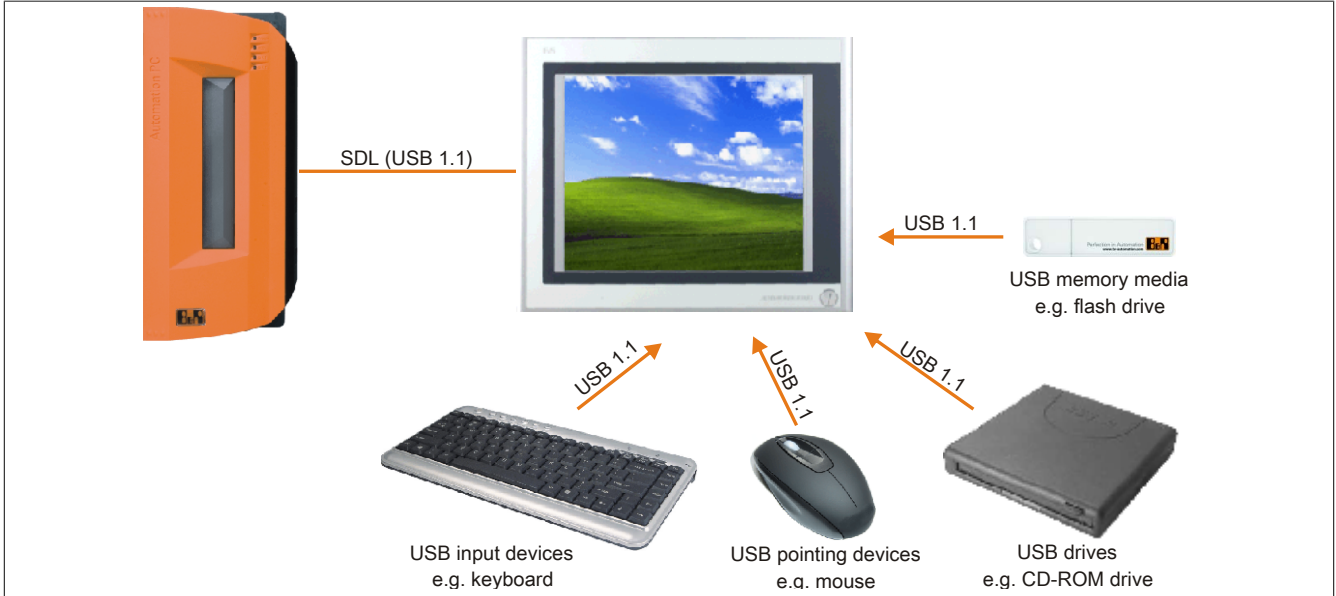
Figure 99: Remote connection of USB peripheral devices on the APC800/900 via SDL
