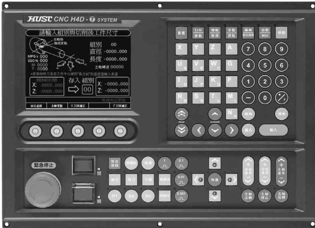
Fig.5-2 Panel of H4D-T Dimensions
