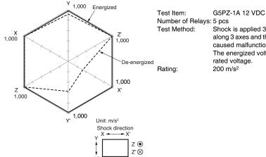
G5P2-1A 12 VDC ys: 5 pcs Shock is applied 3 times in 6 directions along 3 axes and the level at which shock caused malfunction is measured. The energized voltage is 100% of the rated voltage. 200 m/s<sup>2</sup>
