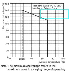
power voltage, not a continuous voltage.
