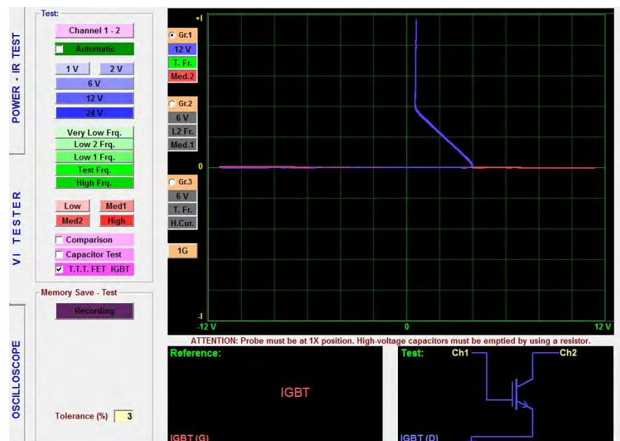
Figure 155: IGBT VI Graph, Equivalent Circuit Diagram
