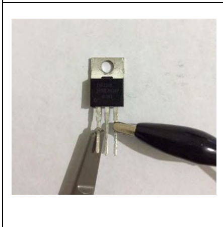
Figure 128: Channel1 Probe Used for Gate - Source Measurement
