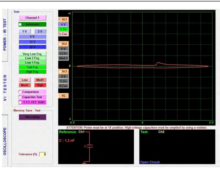
Figure 129: Gate (+) Source (-) VI Graph
