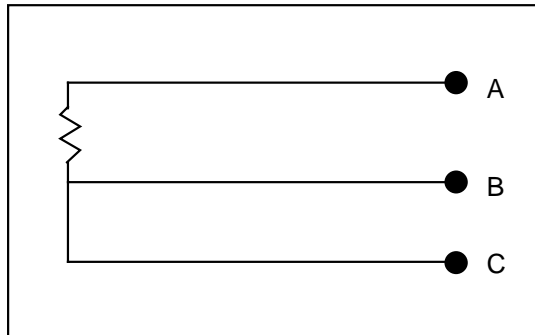
Figure 8-1 RTD Calibration Connection
