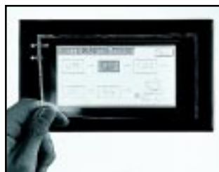
Protective sheet shields display from dirt and scratches
