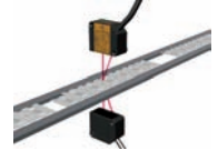
Checking for doubled-up lead frames
