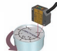
Inspecting pressure indicator dials and pointer gaps
