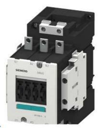
CONTACTOR AC-1, 140 A/400 V, 24 V DC, 3-POLE, SIZE S3, SCREW TERMINAL, WITHOUT BOX TERMINALS LATERAL AUX. SWITCH BLOCK L+ R 2 NO + 2 NC.
