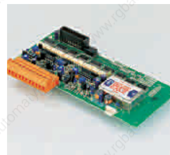
Analogue output board 2 outputs, 10bit resolution
