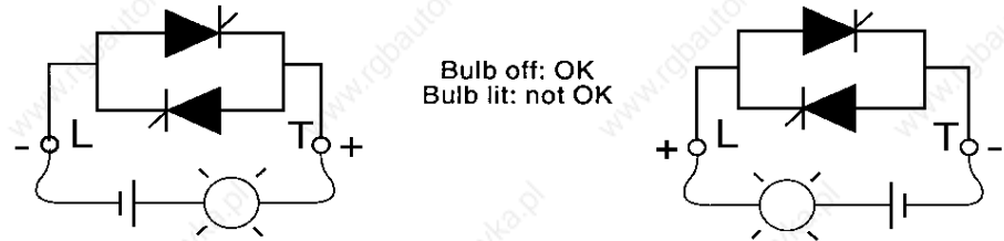
Figure 37 Checking Thyristors
