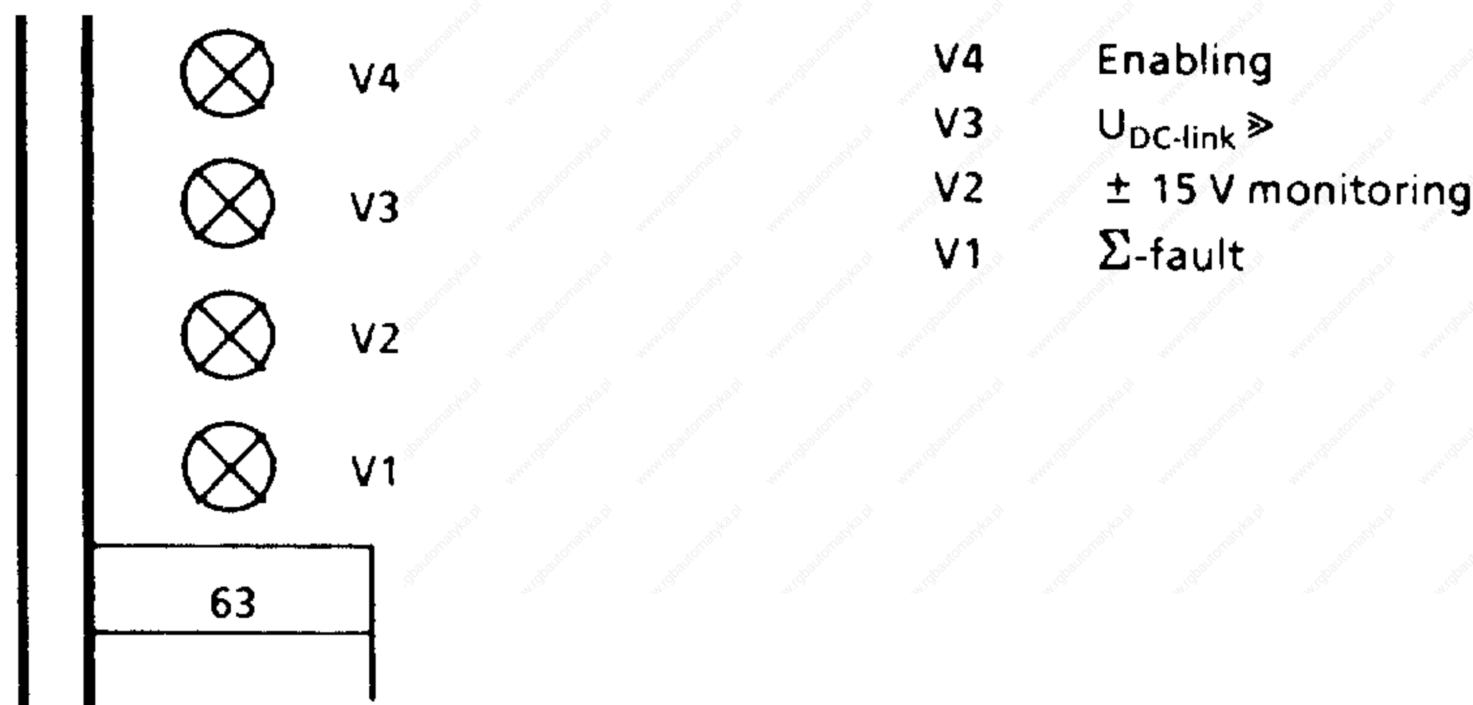
Fig. 3.15 Display elements on power supply module G0
