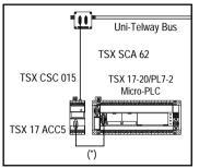
The address coding of a TSX 17-20 Micro-PLC on a Uni-Telway bus is defined by software configuration. The settings of the microswitches located in the subscriber sockets are overridden.
