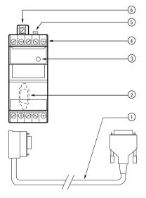
An adapter module (Ref. TSX 17 ACC5) that connects the Micro-PLC to the Uni-Telway bus via the programming port, comprising:
