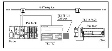
A TSX T407 terminal fitted with the TSX TS4 31 adjustment cartridge and connected to the programming port of the Uni-Telway bus Master PLC can perform adjust and diagnostics functions on the TSX 17-20 PLC and diagnostics on the Uni-Telway bus.
