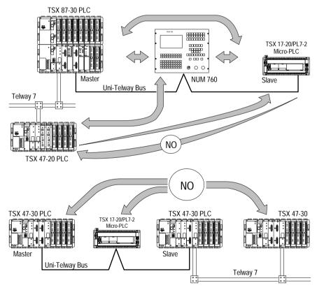
Transparent communications stop when a slave PLC is reached. To go beyond that point communications have to be processed by the application program of the slave PLC.
