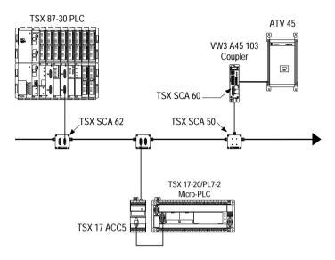
PLC The TSX SCM 21.6 module in the TSX 87-30 is the data link master. The TSX 17 ACC5 Adapter on the TSX 17-20 is a slave. Their application programs, via the text blocks are clients that can:
