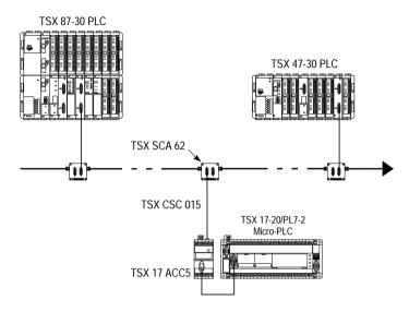
PLCs In the configuration illustrated above, the TSX SCM 21.6 module in the TSX 87-30 PLC is the data link **master**.
