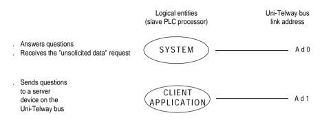
Access to the system gate is always available through address Ad0. This address is defined by configuration.
