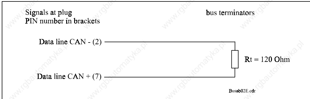
Fig. 48: CAN bus terminators
