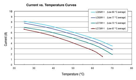
Place test samples in oven at 25 °C, 40 °C, 60 °C and 70°C and increase current flow through the sample at a rate of 0.1 A/minute and record current value when sample trips.
