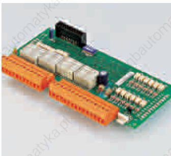
Relay expansion board 12 inputs, 8 relay outputs, 2.0A
