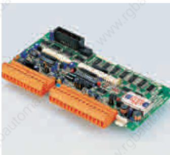
Analogue I/O board 4 inputs/1 output, 8bit resolution
