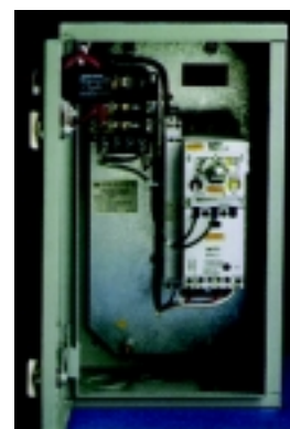
A 30 HP, 460 V self protected combination motor controller: PKZ 2-SP installed in a NEMA 1 enclosure with fused control transformer, extra auxiliary contact and pilot devices
