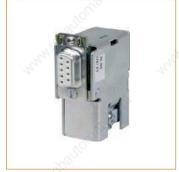
The AC911 bus connector is used to connect a controller to a CAN network. The termination resistor is integrated in the bus connector. The terminating resistor can be turned on or off.
