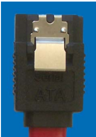
Figure 2-13: CP-HDD-S-KIT SATA Cable - View of Locking Clip
