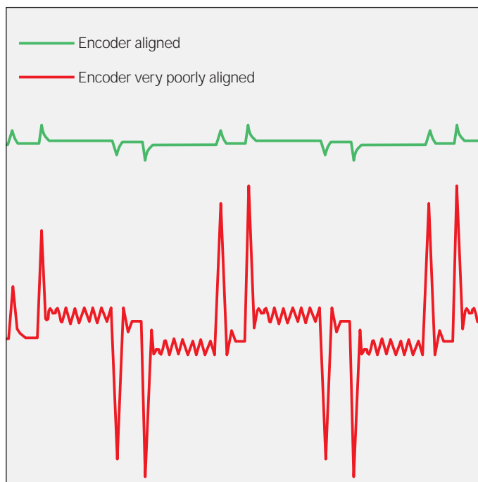
Motor current of adjusted and very poorly adjusted rotary encoder
