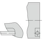
Radial outlet cable connection is not supported by higher accuracy models, modular editions without housings, as well as smaller diameter series like A28 or A36.
