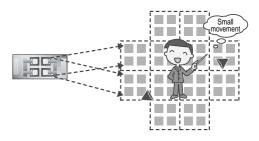
4. Small temperature differences also detected. N a P i 0 n detects the temperature difference between the detection target and its surroundings, and the lowest required temperature difference to the background is  $4^{\circ}$ C  $7.2^{\circ}$ F.
