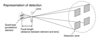
3. Lenses can be miniaturized because the pyroelectric element is small
